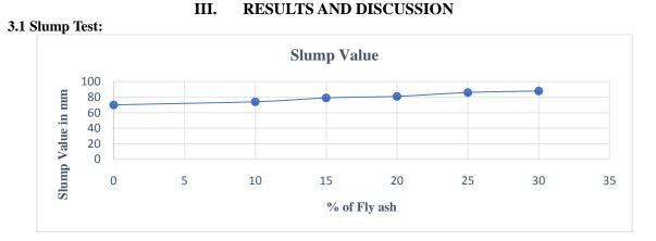
The results show that the slump value increases with an increase in the percentage of fly ash content in the concrete.
